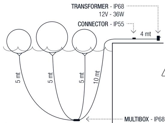
**!** The connector, the transformer and the plug must keep away from the water contact!
