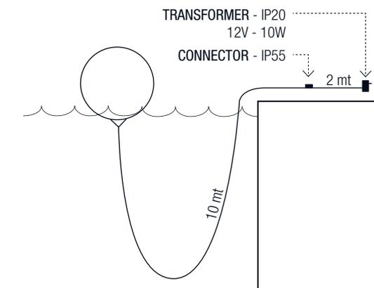
**!** The connector, the transformer and the plug must keep away from the water contact!
